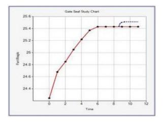
• When the graph does not flatten out consider the 'Pack and Hold' concept
